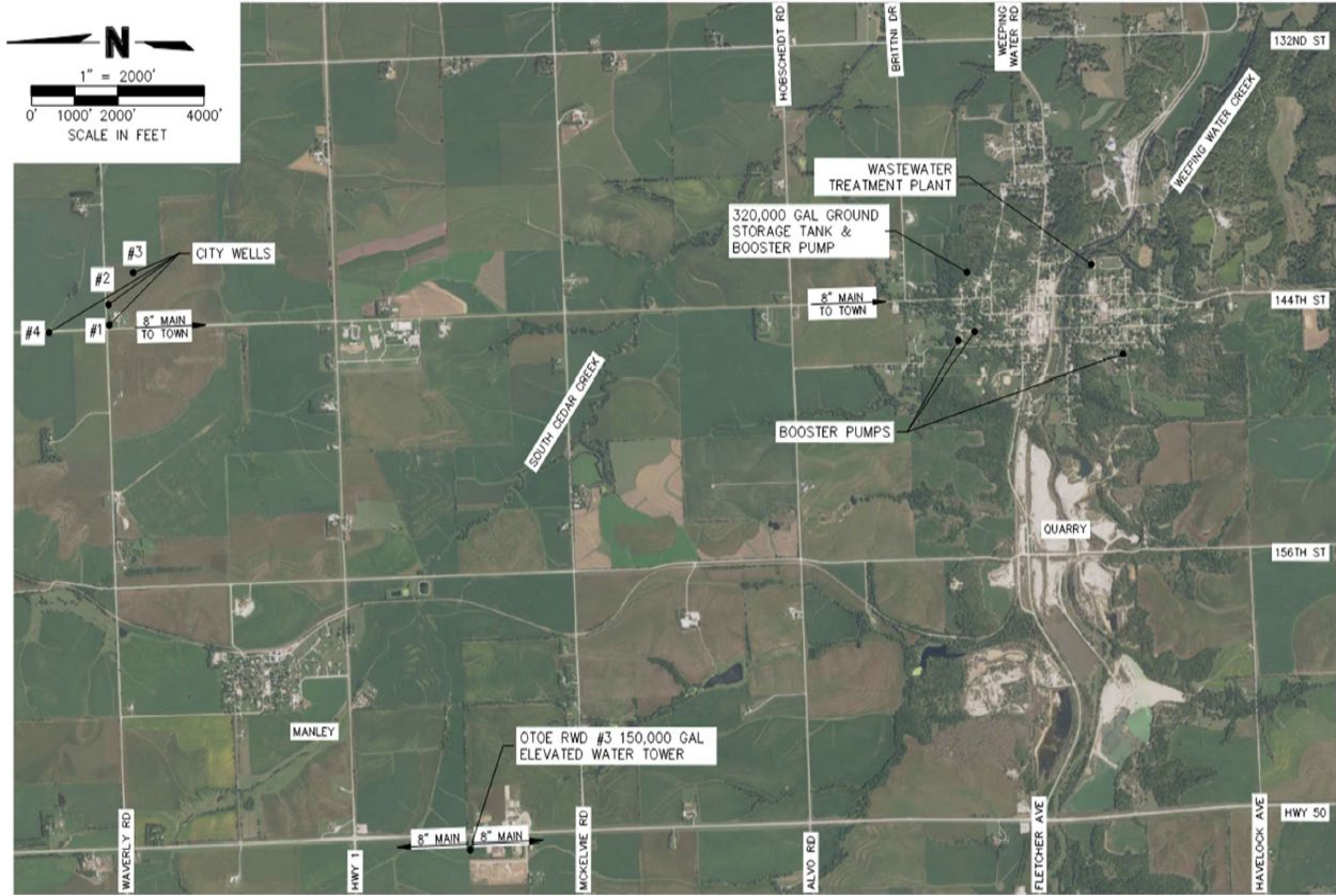
Figure 5. Water System Layout
