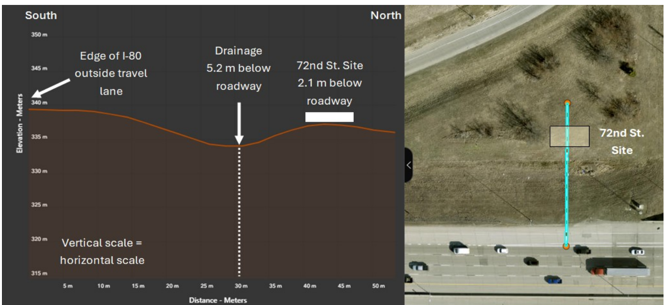
Figure 59. Elevation profile from I-80 outside travel lane through 72nd Street candidate site
