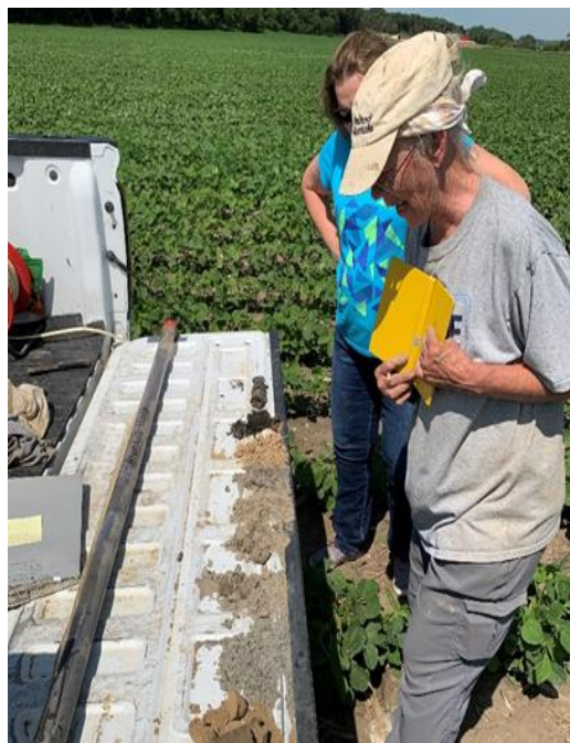
UNL-CSD Hydrogeologist, Susan Olafsen Lackey with LCNRD Office Manager, Marilyn Schumacher evaluating geologic samples collected using a geo-probe from the Missouri River Alluvium near Aten, NE.
